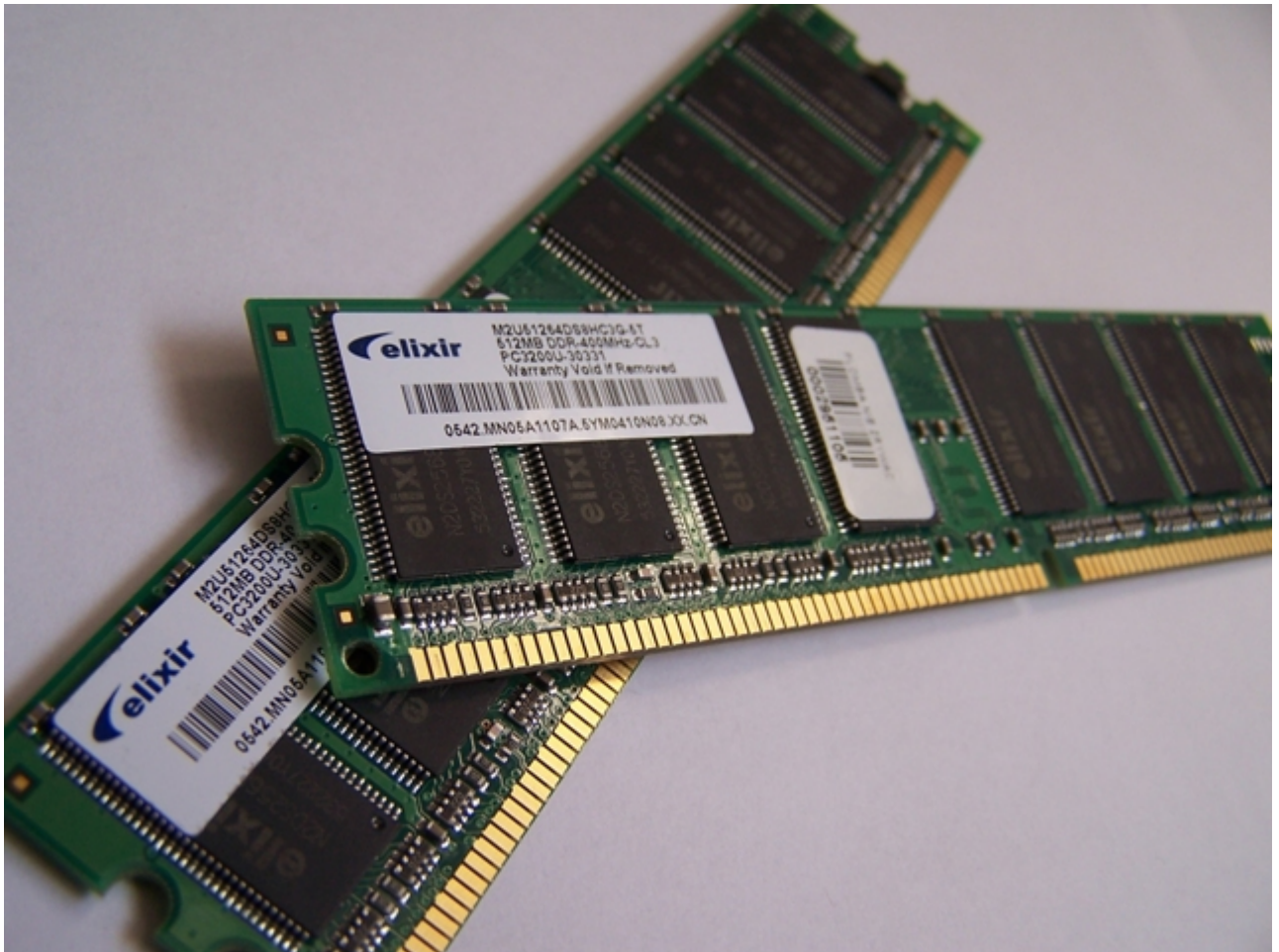
Example of writable volatile random-access memory. Wikimedia Commons.
